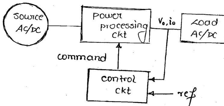
→ Power electronics is a technology associated with efficient conversion & control of electric power, by using power semiconductor devices.
