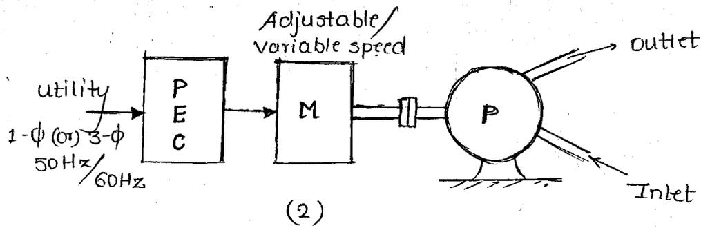
→ In the application, light-fans pumps, compressors & blowers (where  $T_L \propto \omega^2$ ), the overall efficiency of the system can be increased or improved by operating the motor as adjustable or variable speed motors.
