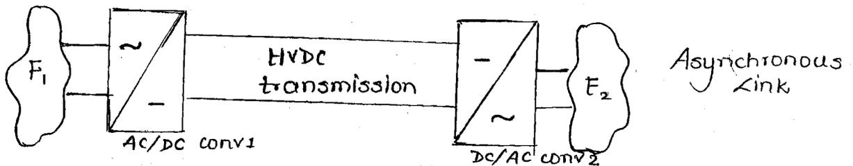
→ HVDC transmission is preferred to connect two ac s/s operating at different frequencies.
